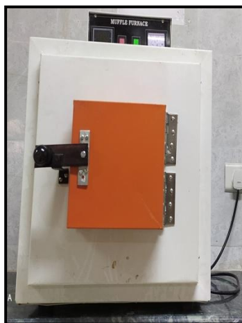
Muffle furnace used for determining the volatile matter and ash content
