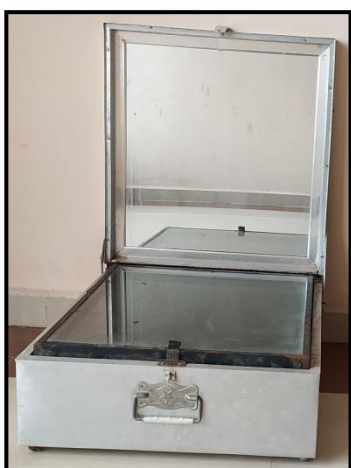
Box type solar cooker used for baking and boiling type of cooking
