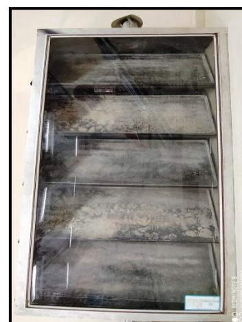
Cabinet solar dryer used for drying of agro products
