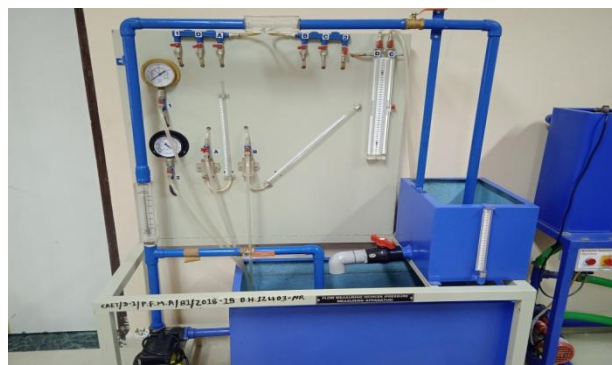
Bernoulli's theorem Apparatus It is used to verify Bernoulli's theorem of fluid flow
