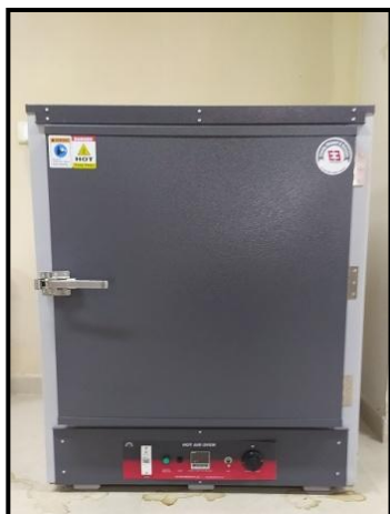
Hot Air Oven used for determining the moisture content and drying purpose
