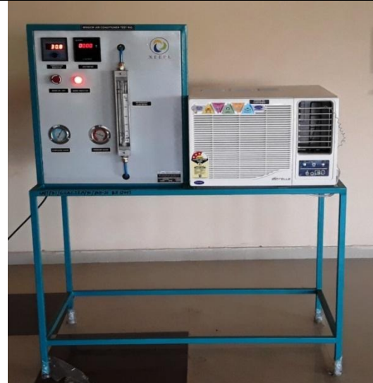
Window Air Conditioner Test Rig It is used to find actual and theritcal coefficient of performance
