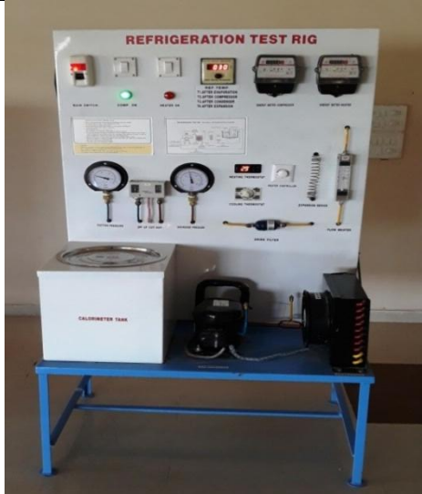
Refrigeration Test Rig It is used to find actual and theritcal coefficient of performance
