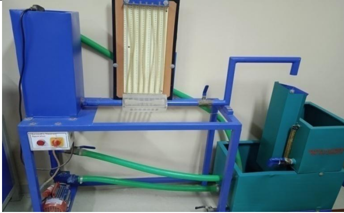
Bernoulli's theorem Apparatus It is used to verify Bernoulli's theorem of fluid flow
