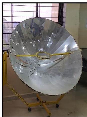
Solar parabolic concentrator cooker used for cooking (boiling and frying type)
