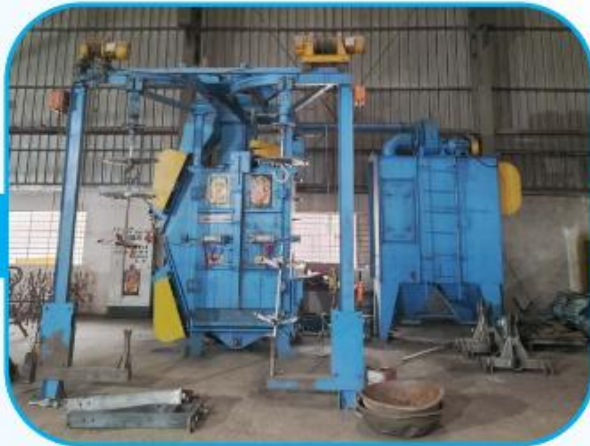
SHOT BLASTING PROCESS
