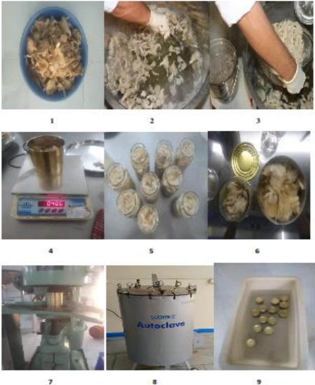
Figure 1: (1) Oyster mushroom, (2) Blanching (3) Water drain from blanched oyster mushroom (4) Weighing (5) Oyster mushroom bottles (6) filling in containers (7) Seaming (8) Retorting (9) Cooling.
