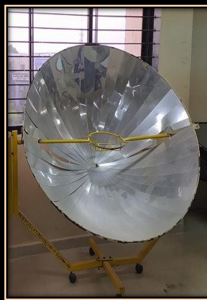
Solar parabolic concentrator cooker used for cooking (boiling and frying type)
