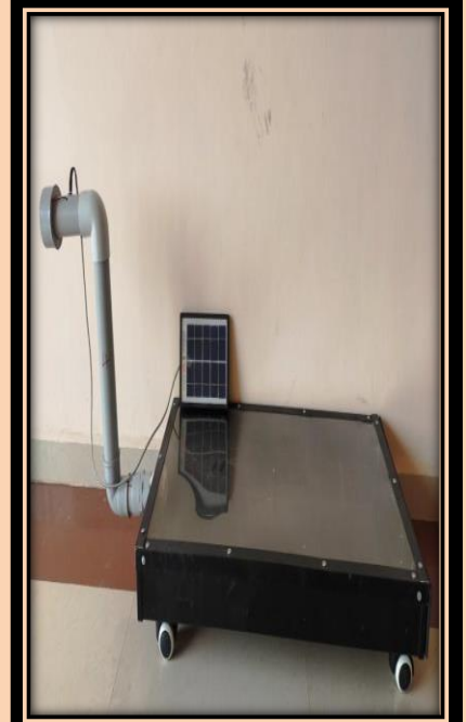
SPV powered baby solar dryer for drying of agro products
