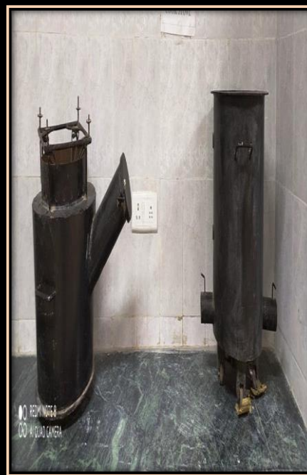
Improved biomass cookstove used for community cooking purpose
