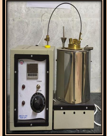
Abel flash point apparatus used for determining the close cup flash point of Petroleum
