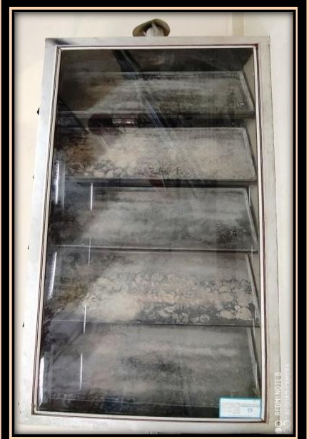
Cabinet solar dryer used for drying of agro products
