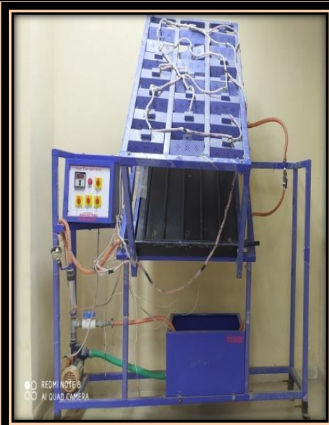
Solar thermal trainer for demonstration purpose and indoor testing of solar collector
