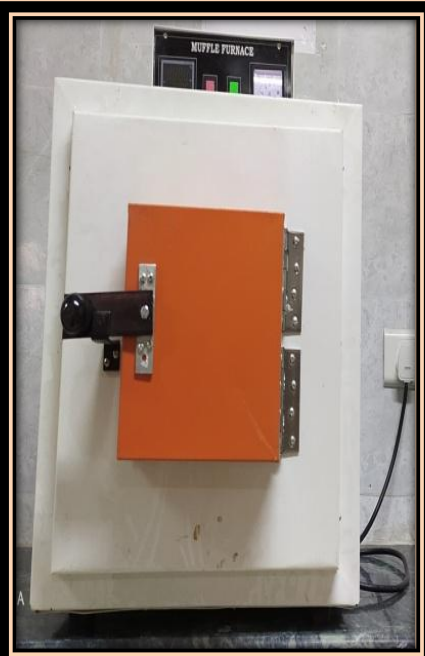
Muffle furnace used for determining the volatile matter and ash content
