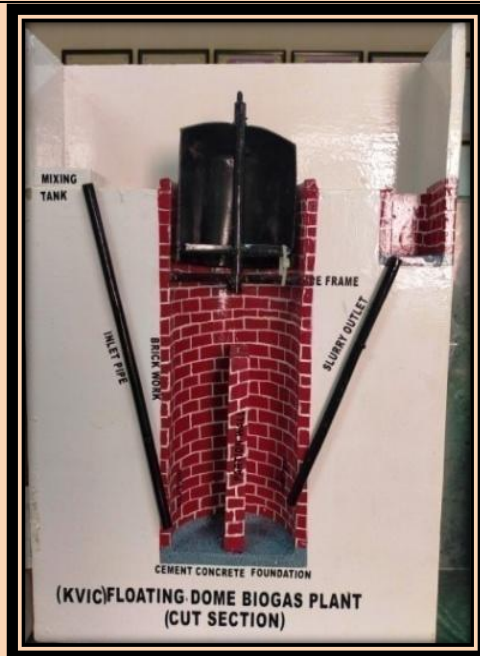
Cut section model of Floating dome biogas plant for practical and demonstration purpose
