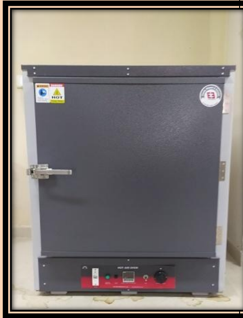
Hot Air Oven used for determining the moisture content and drying purpose
