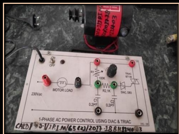
Single Phase AC Power control using DIAC & TRIAC Kit
