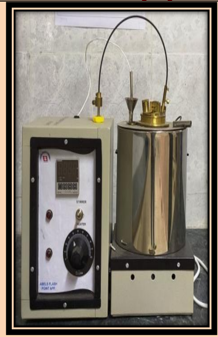
Abel flash point apparatus used for determining the close cup flash point of Petroleum
