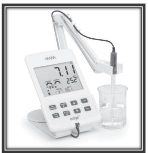
sample solution is determined by dipping the glass electrode in the solution and pH is read directly from the pH meter scale.
