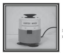
**5.** *Vortex Mixture* - It is also used to mix the reagents during microbiological assay by vortex effect.
